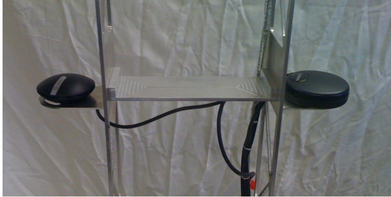
Figure 3: Dual GPS Receivers Mounted on Mast
